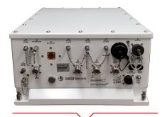
This Narda-MITEQ series of outdoor, antenna-mounted block upconverter is designed to cover simultaneously multiple wide bandwidth satellite transponders by accepting four independent IF inputs which are up converted into one wideband RF output.
