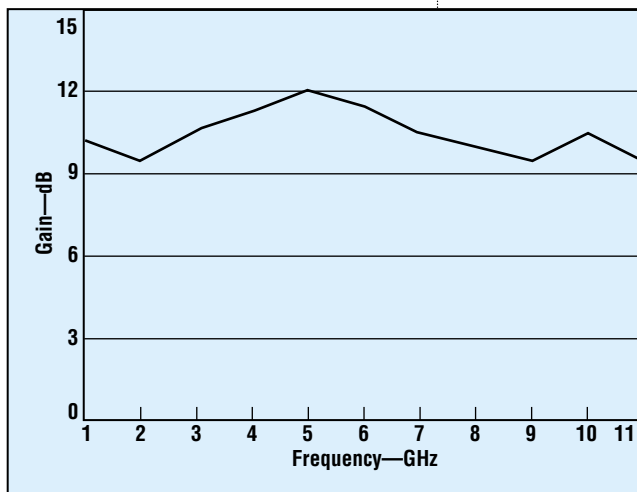
2. The 3-dB bandwidth of the MDD fiber-optic links is 1 to 11 GHz.
